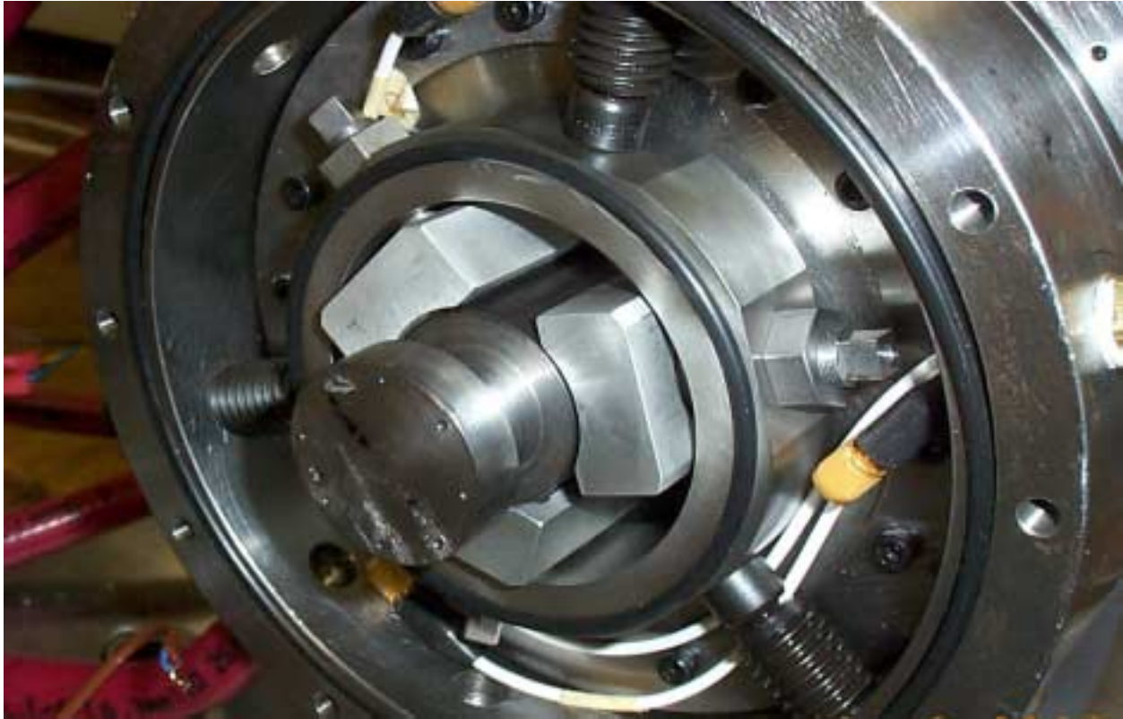
Figure 7. Detail view of HyPad bearing installed in rig
